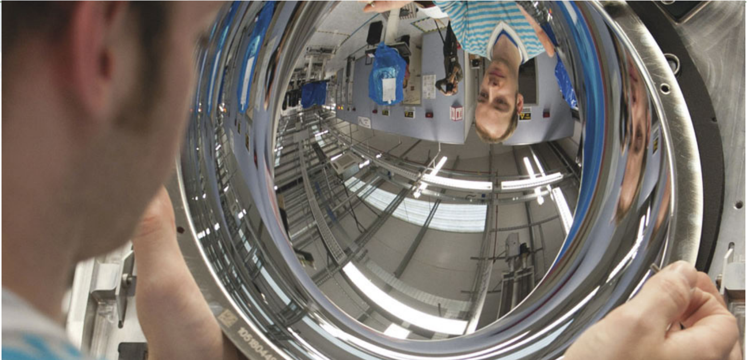
THE ELLIPSOIDAL MIRROR USED BY GLASGOW UNIVERSITY IN THE OPTOS PROJECT.
